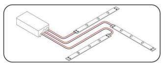
(4) In the 'Array' option, light strip individually powered. Total wattage should be determined so as not to overload power supply. '阵列'接线, 灯条是单独供电的。这种接线方式应确定总瓦数, 以便不要让电源过载。
