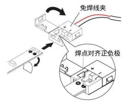
按照灯条上裁剪标识剪裁所需要的长度。将灯条卡入免焊夹中。再合上铰链夹。 Peel away a portion of the light strip adhesive backing at one end. With the solderless clamp open, slide the strip end all the way into the solderless clamp. Close the hinged clamp.
