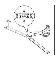
Cut along the light strip tape wherever a dashed line divides two sets of positive and negative connection points.
