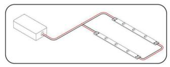
③Light strips are powered from a single looped 'Loopback' connection, which also produces more consistent results. Often used for room perimeter and cove
