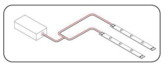
②Light strips are powered from a spliced 'Centerfeed' connection. This type of layout tends to produce more consistent brightness and color between strips.
