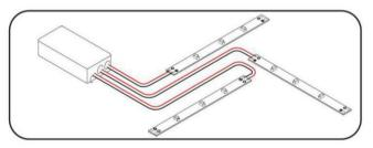
In the 'Array' option, light strip 'legs' are individually powered. Total wattage should be determined so as not to overload power supply.
