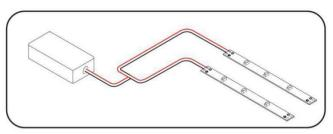
@Light strips are powered from a spliced 'Centerfeed' connection. This type of layout tends to produce more consistent brightness and color between strips. 灯带'并联'再连接电源。这种接线方式更有利于在条带点亮后拥有一 致的亮度和颜色。
