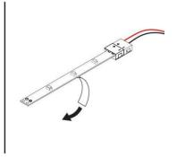
表面,再连接电源。 Remove the remaining adhesive backing and attach the light strip to the desired surface.
