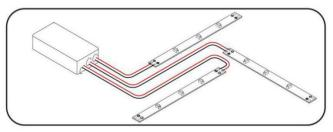
(4) In the 'Array' option, light strip individually powered. Total wattage should be determined so as not to overload power supply. '阵列'接线, 灯条是单独供电的。这种接线方式应确定总瓦数, 以便不要让电源过载。
