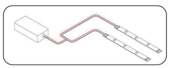
@Light strips are powered from a spliced 'Centerfeed' connection. This type of layout tends to produce more consistent brightness and color between strips.
