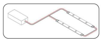
3 Light strips are powered from a single looped 'Loopback' connection, which also produces more consistent results. Often used for room perimeter and cove
