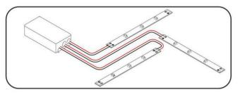
(4) In the 'Array' option, light strip 'legs' are individually powered. Total wattage should be determined so as not to overload power supply.
