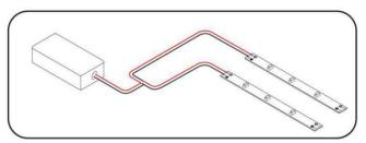
@Light strips are powered from a spliced 'Centerfeed' connection. This type of layout tends to produce more consistent brightness and color between strips.
