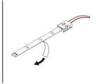
表面,再连接电源。 Remove the remaining adhesive backing and attach the light strip to the desired surface.
