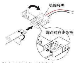
Peel away a portion of the light strip adhesive backing at one end. With the solderless clamp open, slide the strip end all the way into the solderless clamp. Close the hinged clamp.
