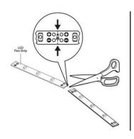
按照灯条上裁剪标识剪裁所需要的长度。将灯条卡入免焊夹中。再合上铰链夹。 Cut along the light strip tape wherever a dashed line divides two sets of positive and negative connection points.
