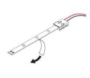
撕下双面胶把灯条粘贴在所需位置 表面,再连接电源。 Remove the remaining adhesive backing and attach the light strip to the desired surface.
