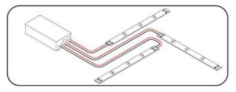
(4) In the 'Array' option, light strip 'legs' are individually powered. Total wattage should be determined so as not to overload power supply.
