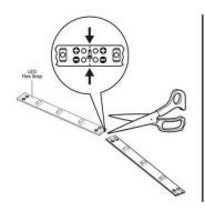
按照灯条上裁剪标识剪裁所需要的长度。 Cut along the light strip tape wherever a dashed line divides two sets of positive and negative connection points.
