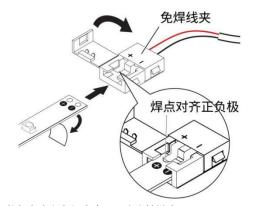
将灯条卡入免焊夹中。再合上铰链夹。 Peel away a portion of the light strip adhesive backing at one end. With the solderless clamp open, slide the strip end all the way into the solderless clamp. Close the hinged clamp.
