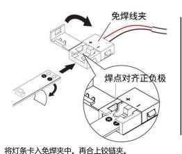
Peel away a portion of the light strip adhesive backing at one end. With the solderless clamp open, slide the strip end all the way into the solderless clamp. Close the hinged clamp.
