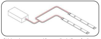
②Light strips are powered from a spliced 'Centerfeed' connection. This type of layout tends to produce more consistent brightness and color between strips. 灯带'并联'再连接电源。这种接线方式更有利于在条带点亮后拥有一致的亮度和颜色。
