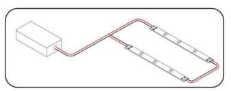
③Light strips are powered from a single looped 'Loopback' connection, which also produces more consistent results. Often used for room perimeter and cove
