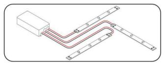
④In the 'Array' option, light strip 'legs' are individually powered. Total wattage should be determined so as not to overload power supply. '阵列'接线, 灯条是单独供电的。这种接线方式应确定总瓦数,以便不要让电源过载。
