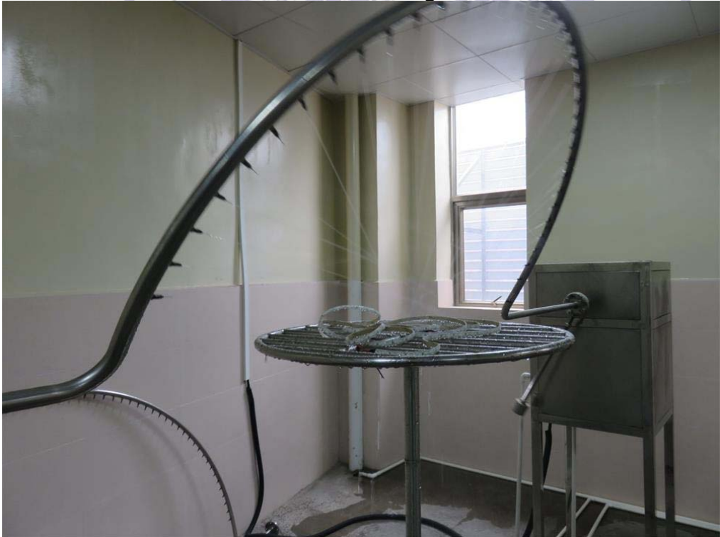
Photo 8 IPX4 Testing view
