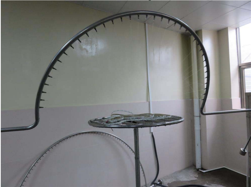
Photo 7 IPX4 Testing view
