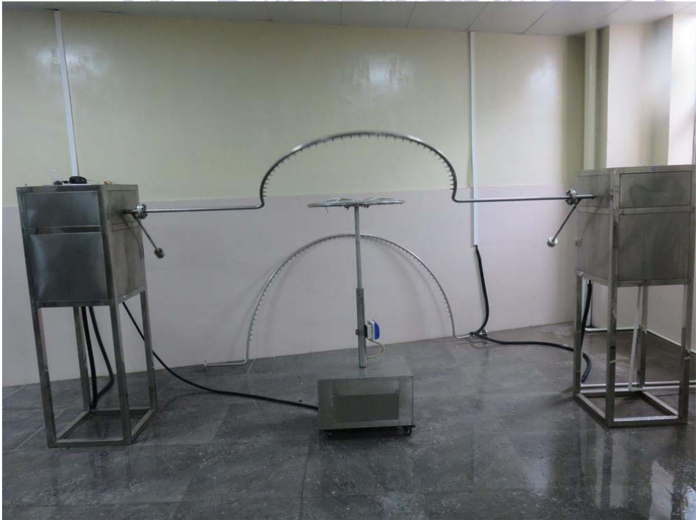
Photo 6 IPX4 Before testing view
