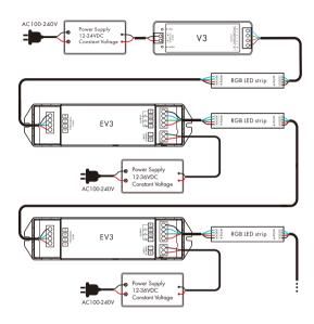
Note: If the power repeater is over heat or short circuit, the LED indicator will blink.
